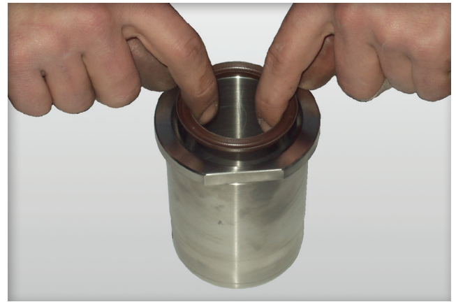
04 Place the gaskets support unit on a clean surface and pull the gaskets out (item 3).
